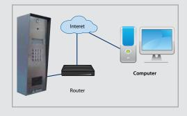
Remote PC via (optional) DSL modem or IP module
